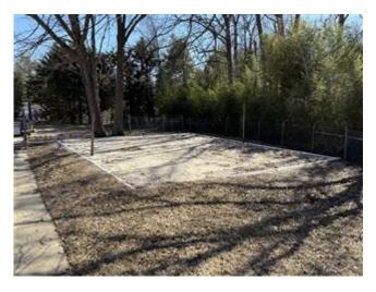
**Tot Lots.** The community maintains one tot lot. The tot lot includes a swing set, wood/synthetic borders, a wood chip surface, and a tether ball pole. The facility appears to be in generally good condition, with no noted wear, loose connections, cutting, entanglement, or falling, but with potential tripping hazards. The wood chip surface does not appear to be adequate. We noted that the swing set is installed on a slope.
